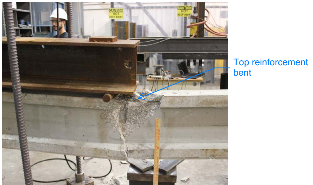
Figure 10. Beam at failure (flexure).
